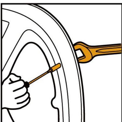
Tighten the valve by wrench and screw it ( Torque value must be  $\geq 4\text{Nm}$ )
